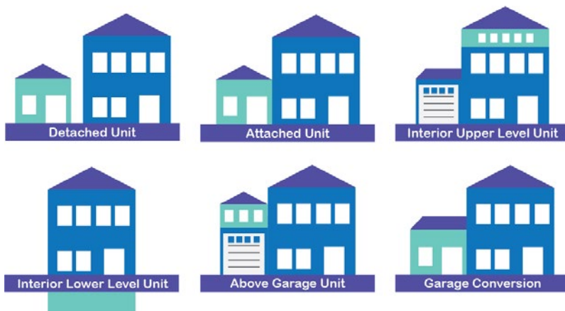
Figure 4-2. Illustration depicting different types of accessory dwelling units (by Cole Jackson, licensed by CC BY 1.0)
